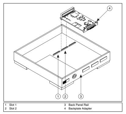
Figure 1. Installing the SB-GPIB/TNT or SB-GPIB
